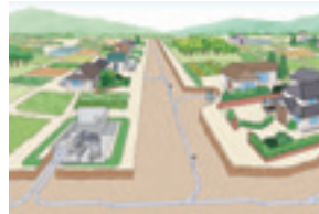
Vacuum sewerage system
