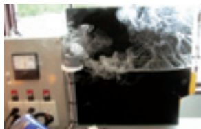
Simulating a fire resulting from excessive electrical current due to plugging too many devices into a single outlet
