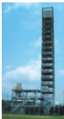
Eslon Tower (Test equipment for pipelines for buildings)
