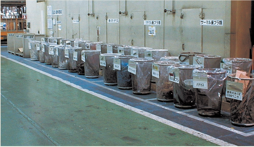
Segregated waste station at the production line where clear plastic bags are provided to make distinction easy.
