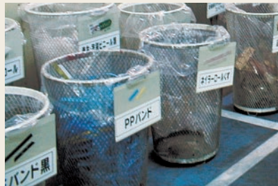
Segregated waste station at the production line where clear plastic bags are provided to make distinction easy.
