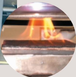
■ Cone Calorimeters ISO-5660 (Heat volume, heat speed) Size of test piece: 100 x 100 mm ● Uses: Noncombustible trials, semi-noncombustible trials, fire resistance trials
