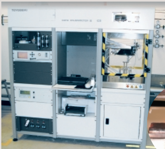
■ Cone Calorimeters ISO-5660 (Heat volume, heat speed) Size of test piece: 100 x 100 mm ● Uses: Noncombustible trials, semi-noncombustible trials, fire resistance trials
