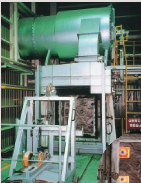
■ Vertical furnace JIS A 1302 (Grade 2 fire protection) JIS A 1304 (1 hour fire resistance) ISO-834 (1 to 2 hours of fire protection and resistance) Effective heat area: 1000 x 1000 mm ● Uses: Walls, fireproof doors, under eaves, sashes
