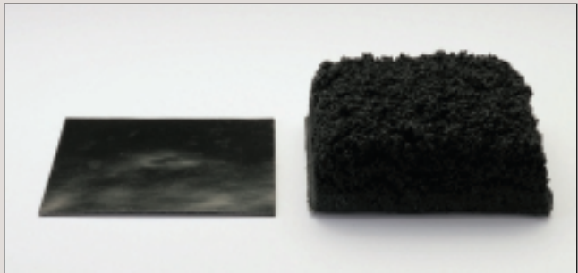
Example:The epoxy "Fi-Block "expands roughly 30 times.
