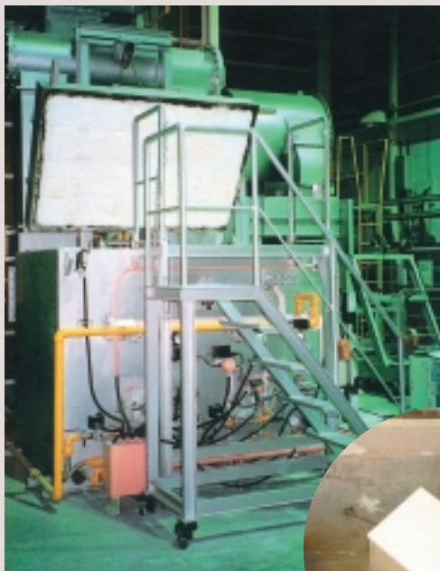
■ Horizontal furnace JIS A 1302 (Grade 2 fire protection) JIS A 1304 (1 hour fire resistance) ISO-834 (1 to 2 hours of fire protection and resistance) Effective heat area: 1000 x 1600 x 1300 (H) mm ● Uses: Columns, beams, floors, roofs
