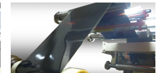
Roll-to-roll production of film-type perovskite solar cells
