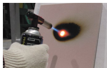
Certified non-combustible, heat-insulating urethane foam for on-site use
