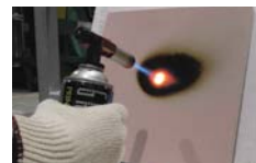
Non-combustible certified material, thermal insulating urethane foam material for onsite use
