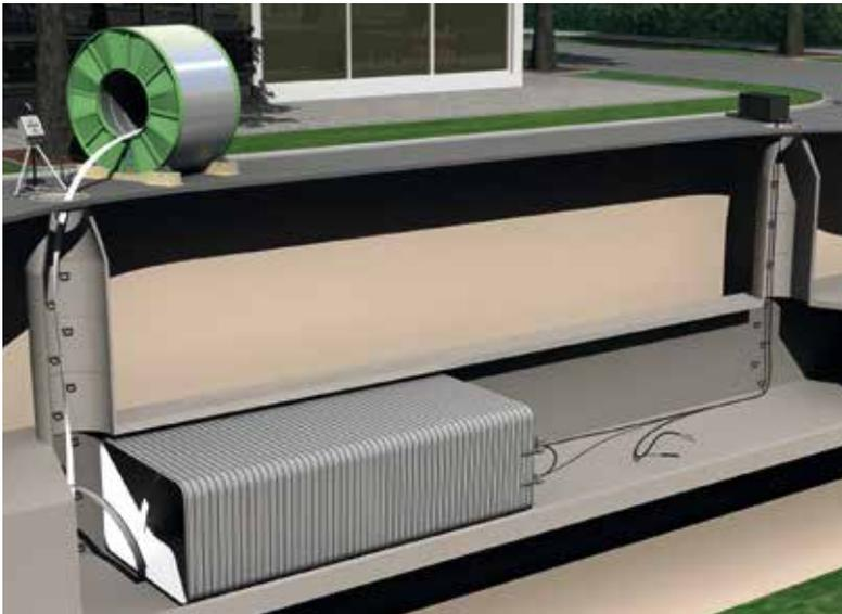
SEKISUI Pipe Renewal stands for technological competence in trenchless pipe rehabilitation with spiral-wound linings. We manufacture the profiles and offer all services for successful realisation of your rehabilitation projects.
