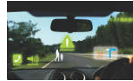
New head-up display system that is capable of displaying information over the entire windshield
