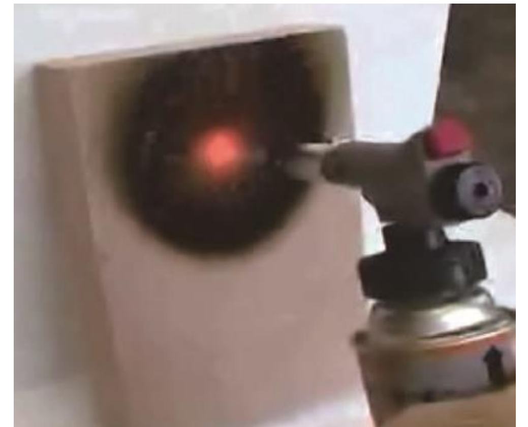
Thermal insulating urethane foam material for onsite use
