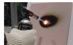
Non-combustible certified material, thermal insulating urethane foam material for onsite use
